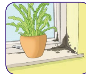
mould and damp
